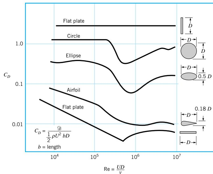
■ **FIGURE 9.22** Character of the drag coefficient as a function of Reynolds number for objects with various degrees of streamlining, from a flat plate normal to the upstream flow to a flat plate parallel to the flow (two-dimensional flow) (Ref. 5).
